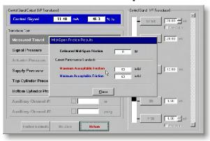
A functional, intuitive calibration tool provides accurate and efficient setup of the control valve. BenchMark communicates with either analog or digital valves. Friction can be quickly evaluated at mid-span for the proper adjustment of packing pre-
